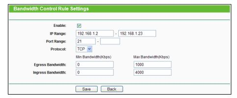
Figure 4-103 Bandwidth Control Rule Settings
